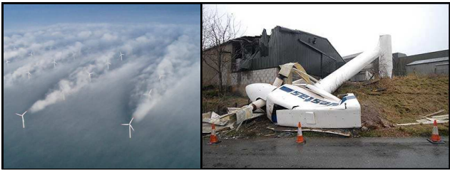
Figure 1: (a) The wake field of a wind farm decreases performance of down-wind turbines, and (b) turbine failure caused by a combination of high winds and control system failure.
